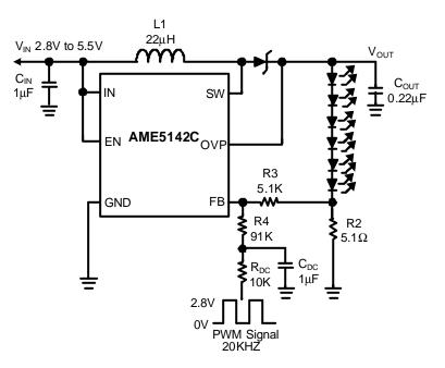
Figure 7. Dimming Control Using a Filtered PWM Signal
