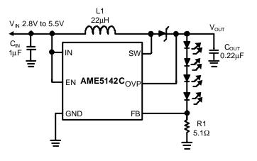
Figure 2: Circuit For Driving 4 White LEDs
