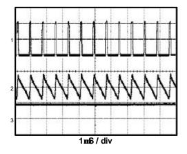
V<sub>IN</sub> = 2.8V; 6 LEDs I<sub>OUT</sub> = 20mA
