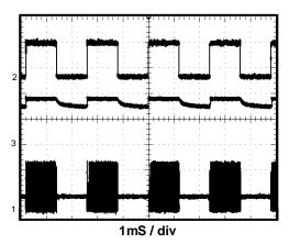
V<sub>IN</sub> = 5.5V; 6 LEDs  $I_{OUT} = 20 \text{mA}$
