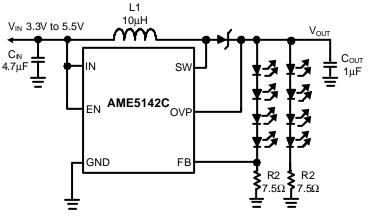
Figure 12: Circuit For Driving 2 Strings of 4 White LEDs
