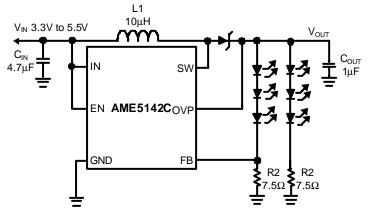
Figure 9: Circuit For Driving 2 Strings of 3 White LEDs
