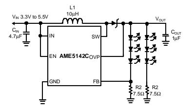
Figure 10: Circuit For Driving 2 Strings of 3 White LEDs
