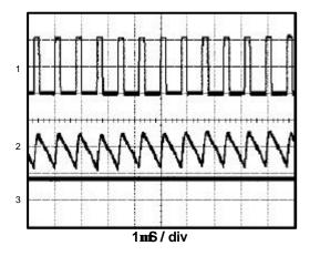
$V_{IN} = 5.5V$ ; 6 LEDs  $I_{OUT} = 20 \text{mA}$
