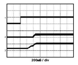
$V_{IN}$  = 2.8V; 6 LEDs  $I_{OUT}$  = 20mA
