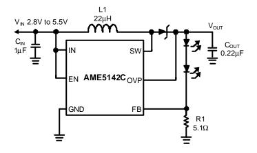
Figure 1: Circuit For Driving 2 White LEDs
