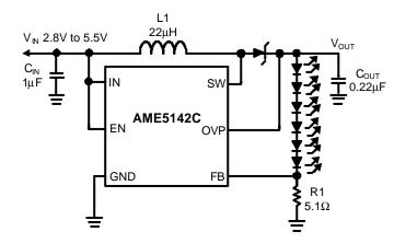
Figure 3: Circuit For Driving 6 White LEDs
