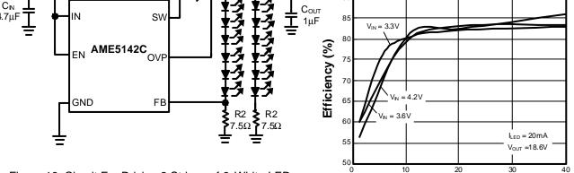
Figure 16: Circuit For Driving 2 Strings of 6 White LEDs
