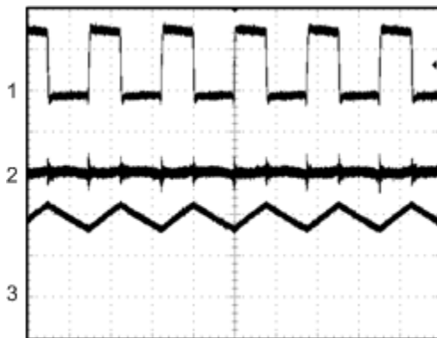
Heavy Load Mode Output Voltage Ripple
